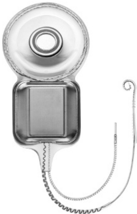
Figure 11.1 Internal part of cochlear implant (Cochlear N512).
