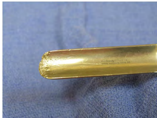
Fig. 5. Retractors and suction tips get damaged during surgery with rotary instruments. Note the sharp edge of the Austin retractor. Unnecessary trauma to reflected tissues can result when faulty equipment goes undetected.
