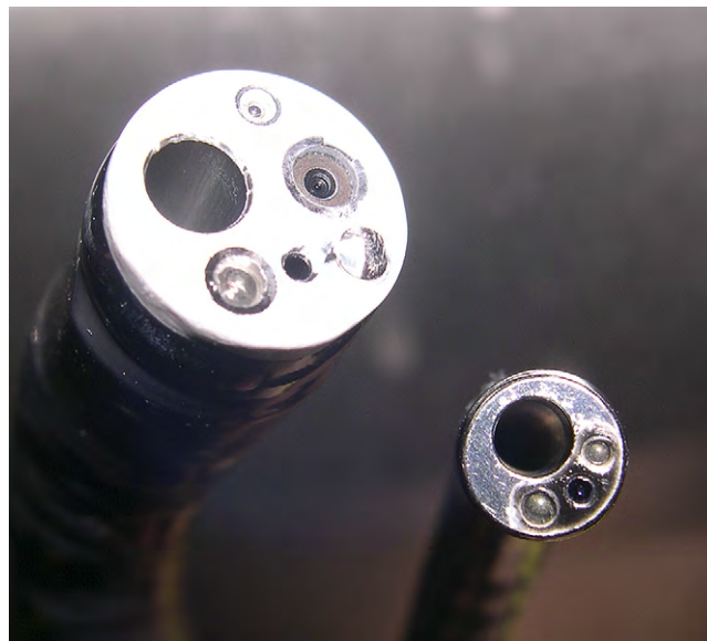
Fig. 2. Large diameter and small diameter endoscope. The larger scopes are most commonly used for large cavity endoscopy, such as bronchoscopy or colonoscopy. Note the instrument channel and the suction port. The smaller diameter scope does not contain an instrument port but may contain a suction port.
