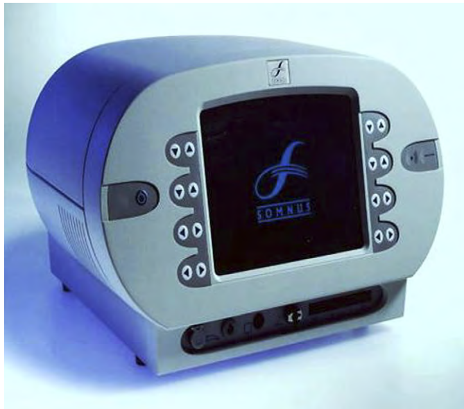
Fig. 1. The Somnus radioablation unit consists of a programmable generator with temperature and impedance monitoring and a disposable surgical handpiece. This was the first US Food and Drug Administration–approved unit specifically for treatment of sleep apnea. (Courtesy of Gyros ENT, LLC, Bartlett, TN; with permission.)
