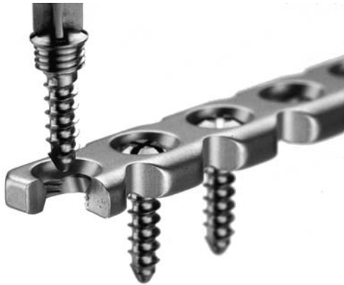
FIGURE 20-13 A locking plate–screw system. Note the second set of threads just under the head of the screw that will lock into receptacle threads inside the hole of the bone plate.
