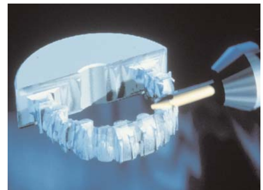
FIGURE 13-51 By entering scanning information into a computer bank, computerized lathes with precisely controlled cutting heads attack the titanium blank to create the milled bar structure.
