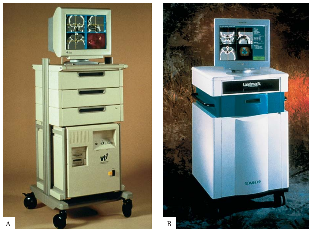
FIGURE 16-16 A and B, Devices for intraoperative stereotactic navigation. A selected point is identified in the coronal, sagittal, and axial planes using reconstructed computed tomographic data. Reproduced with permission from Kennedy DW. Functional endoscopic sinus surgery: concepts, surgical indications, and instrumentation . In: Kennedy DW, Bolger WE, Zinreich SJ, editors. Diseases of the sinuses: diagnosis and management . Hamilton: BC Decker Inc; 2001. p. 206.
