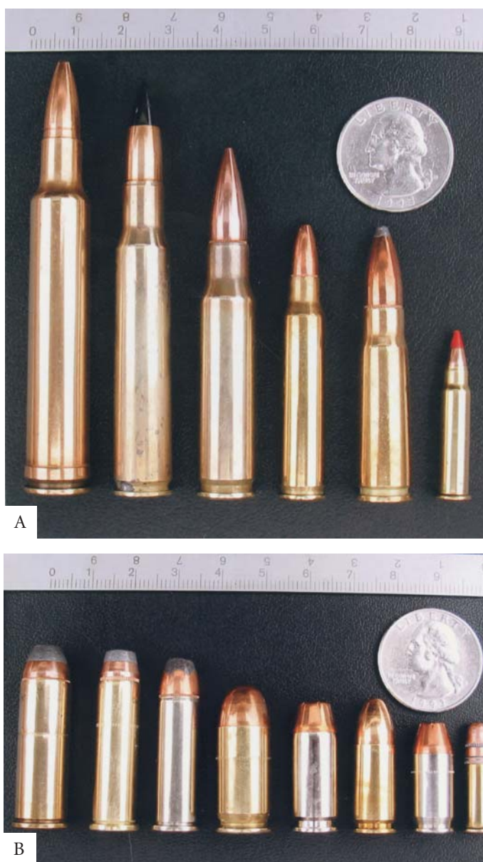
FIGURE 26-1 A, Representative rifle cartridges. From left to right: .300 Winchester magnum, 30-06, .308 (7.62 × 51 NATO), .223 (5.56 × 45 NATO), 7.39 (AK-47 round), and .17 rimfire. B, Representative pistol cartridges. From left to right: .44 magnum, .357 magnum, .38 special, .45 auto, .40 auto, 9 mm auto, .380 auto (9 mm short), .22 rimfire.
