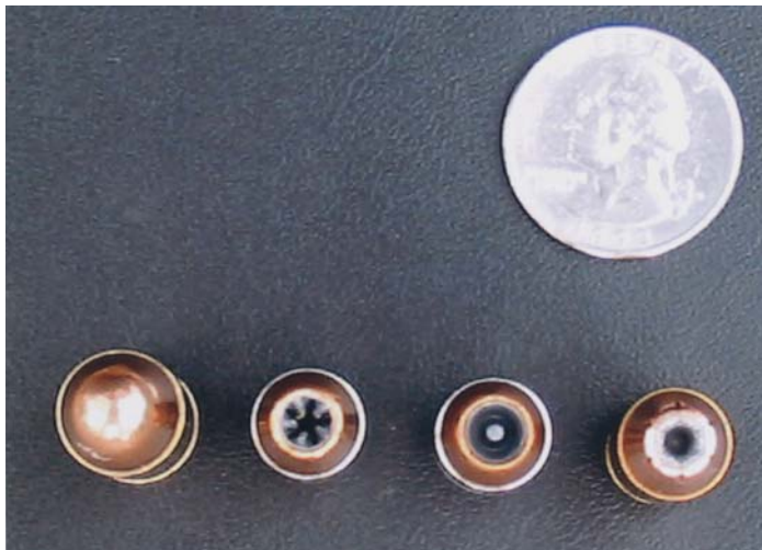
FIGURE 26-4 Full-jacketed bullet compared with various hollow-point rounds designed to aid the expansion of lower-velocity bullets.
