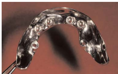
FIGURE 13-52 The milling process is completed at the fit surfaces with a very precise secondary cutting tool that creates fit tolerances in the range of single digit microns. These frameworks are very lightweight and fit with a degree of precision that is difficult to duplicate with conventional casting procedures.
