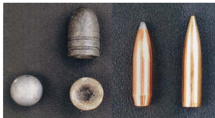
FIGURE 26-3 Left, Early round projectile and Minié ball with expanding base. Right, Modern full-jacketed and soft point rounds with “boat tail” to improve flight characteristics.
