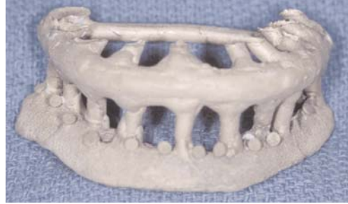
FIGURE 13-46 For greatest accuracy, the casting technique for these long-span restorations usually requires a runner bar and multiple sprue attachments to minimize distortion.
