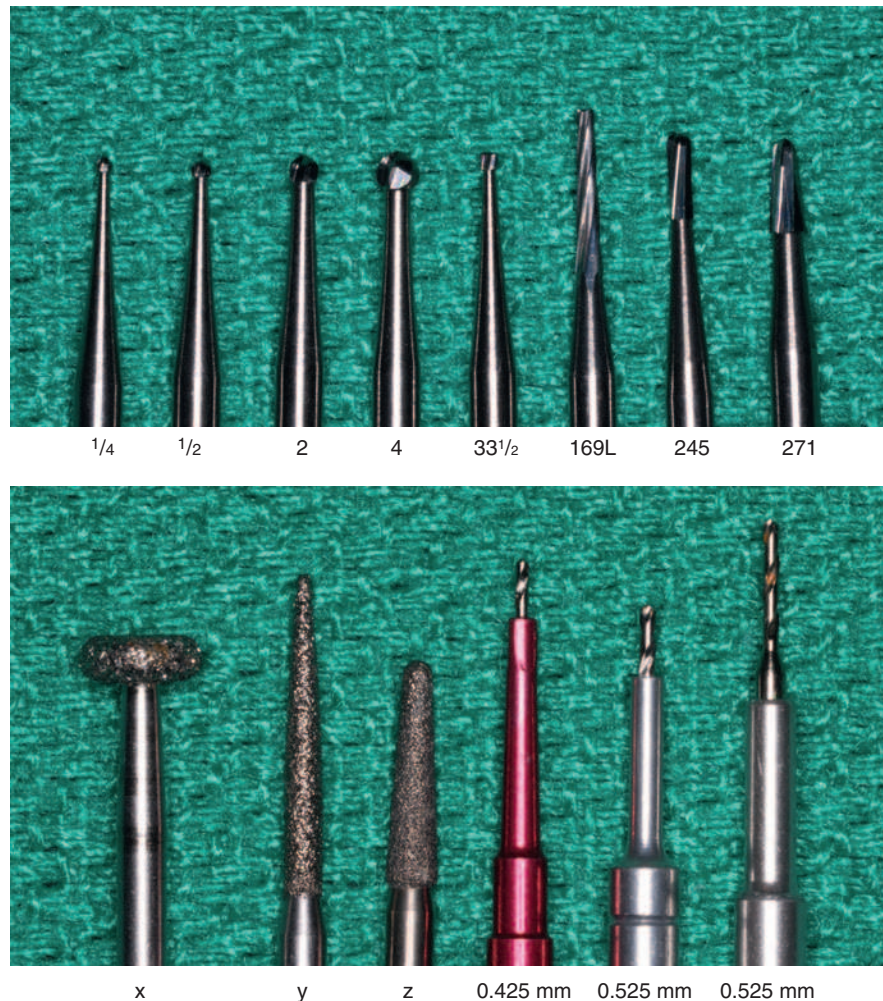
• Fig. 14.21 Burs used in recommended procedures. Bur sizes \frac{1}{4} , \frac{1}{2} , 2, 4, 33\frac{1}{2} , and 169L are standard carbide burs available from various sources. The 245 and 271 burs are nonstandard carbide burs that do not conform to the current American Dental Association (ADA) standard numbering system. They are designed to combine rounded corners with flat ends and are available from several manufacturers. The diamond instruments shown are wheel (x), flame (y), and tapered cylinder (z). Various twist drills are illustrated. Particular drills often are provided as specified by manufacturers of pin-retention systems.
