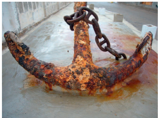
• Fig. 13.8 Example of corrosion due to electrochemical dissolution in water.
