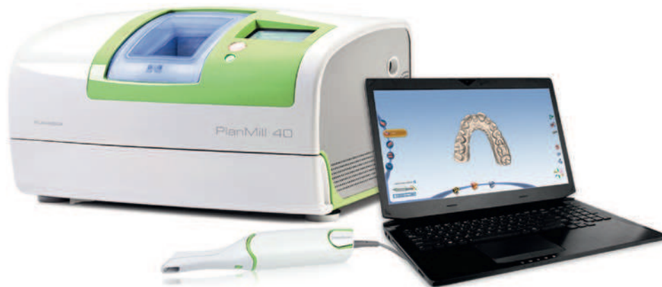
• Fig. 12.2 PlanFit chairside CAD/CAM system. (Courtesy D4D Technologies.)
