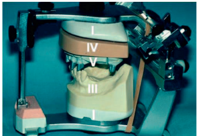
• Fig. 13.57 Cast model showing four types of gypsum products.
