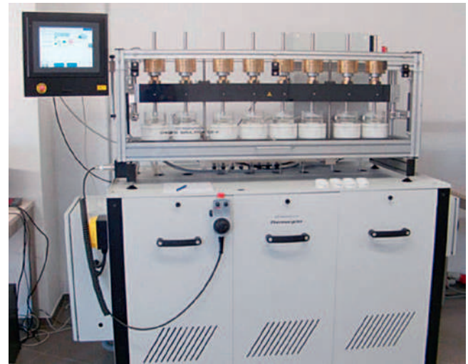
• Fig. 13.13 Eight-chamber chewing simulator.
