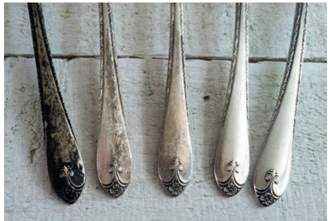
• Fig. 13.7 Tarnish of silverware. Dental alloys may undergo the same discoloration in the oral environment.
