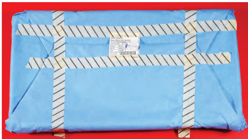
Figure 1.1 A surgical pack after autoclaving. The cross-hatchings on the Bowie-Dick tape have turned brown indicating that the pack has been successfully sterilised.
