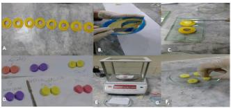
Fig 1A: Split moulds used in study; B. Alginate impression material being mixed in a rubber bowl by spatula; C, Alginate being poured into the moulds; D, Disc shaped samples obtained; E, Measurement
