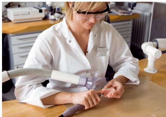
■ Fig. 12.4 Point suction for reducing inhalation of dusts, etc., generated by dental laboratory procedures (Courtesy of E. Østergaard, Århus, Denmark)
