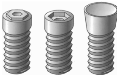
Figure 14-51. External and internal hex and Morse taper connectors. Reprinted with permission from Searson et al. (2005). Copyright © 2005, Quintessence Publishing.
