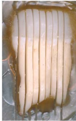
Fig. 3.2. Test assembly for microtensile bond test. (From [1])
