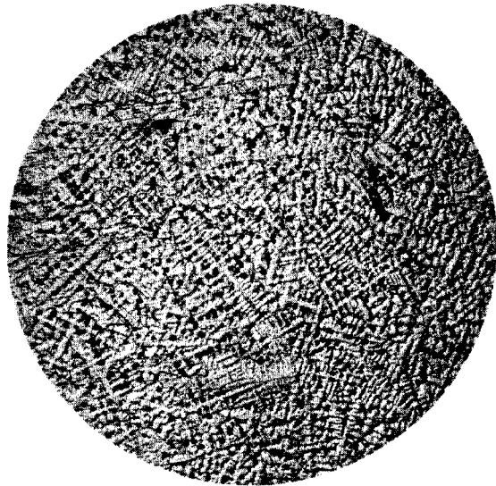
Fig. 6-14 Dendritic structure visible in a low-power light microscopic view of a gold alloy (polished, acid-etched). The treelike branching is similar to that sketched in Fig. 6-13.
