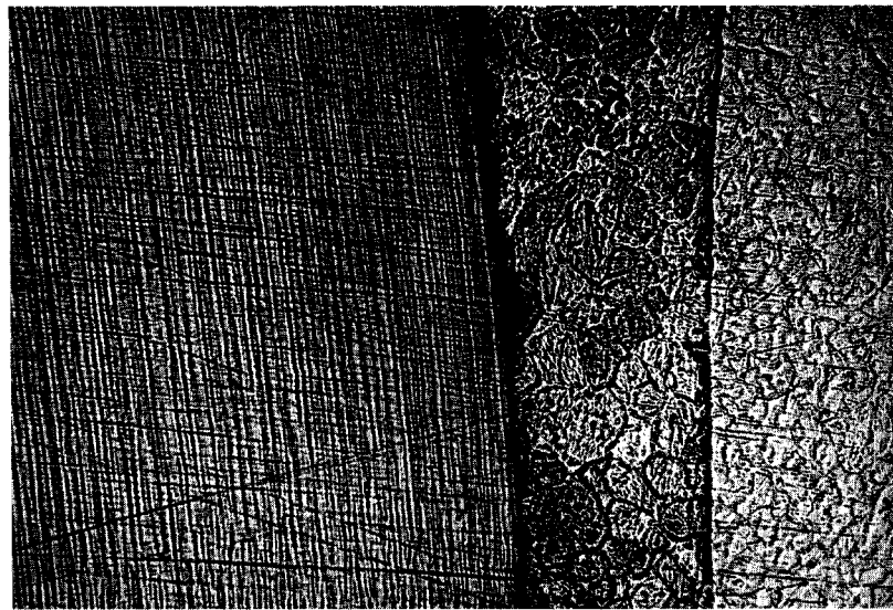
Fig. 15-6 Solder ( middle ) well attached to cast alloy ( right ) but with less satisfactory attachment to the wire ( left ).
