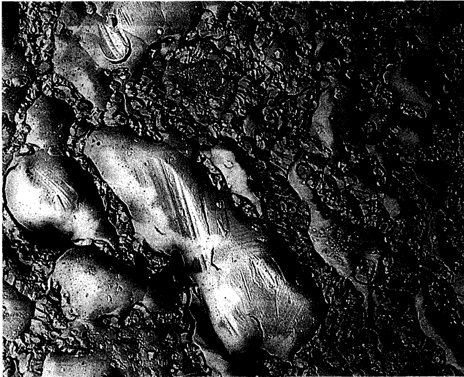
Fig. 19-2 Electron micrograph of replicated oxidized surface of a Au-Pt-Pd alloy ( \times 8000 ). (From Kelly M, Asgar K, O'Brien WJ: J Biomed Mater Res 3:403, 1969.)
