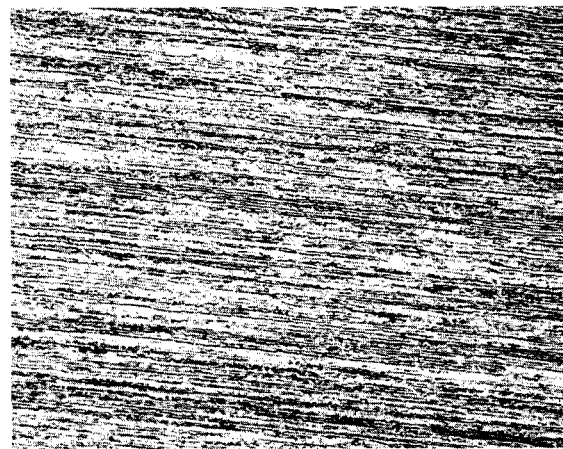
Fig. 6-17 Low-power light microscopic view of a wrought wire microstructure. The grains visible in Fig. 6-16 have been broken apart and tangled among one another. The entangled grains are lined up along the axis of the wire. This type of microstructure is called a fibrous structure for obvious reasons.
