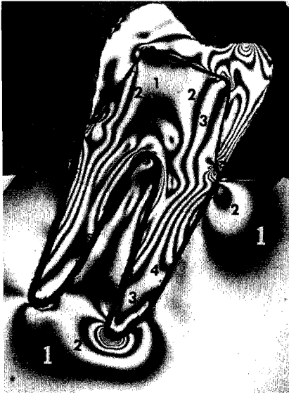
Fig. 4-36 Isochromatic fringes in a two-dimensional photoelastic model of a molar with a full crown under a concentrated force of 266 N; the numbers represent the fringe order of the isochromatic fringes. (From Hood JAA, Farah JW, Craig RG: J Prosthet Dent 34:415, 1975.)
