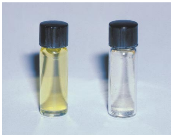
Figure 9-2. These vials show the color of a composite resin before ( left ) and after ( right ) polymerization. Note the shift from yellow to clear that results from polymerization; this color shift resolves roughly 24 hours after curing and greatly affects a restoration's final shade.
