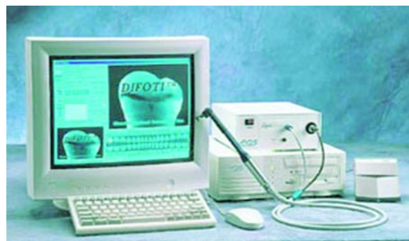
Figure 2–10. The DIFOTI (Electro-Optical Sciences Inc.) uses white light, a CCD camera, and computer-controlled image acquisition and analysis to detect caries.
