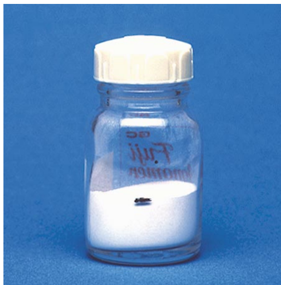
Figure 3-4. A , Glass-ionomer fillers are complex glasses made at high temperature. B , The glass is supercooled in water to produce highly reactive flake-like plates that settle. C , A typical bottle of glass-ionomer powder before and, D , after shaking. Since these materials are dispensed with a scoop, mix accuracy is affected.
