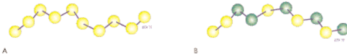
Figure 1–1. A , A linear polymer is made up of multiple units of one type of monomer. B , A copolymer includes more than one type of monomer.
