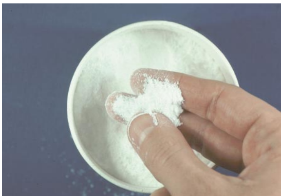
Figure 7-5. The fine silica ash used in microfilled composites. The material is called Airosil and functions as a thickening agent, owing to its small particle size; it is also used to thicken toothpastes, cosmetics, paints, and other household materials.
