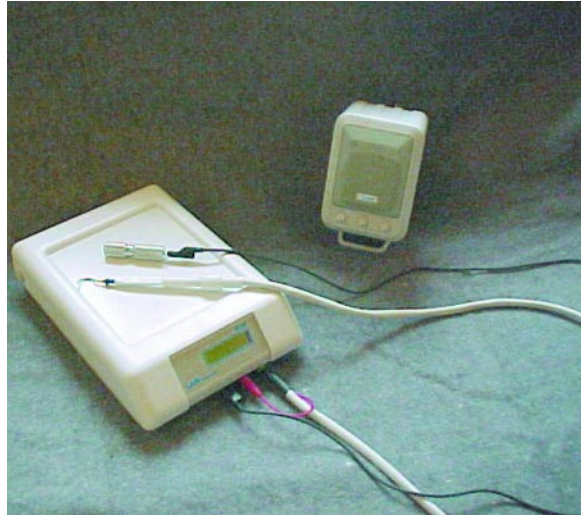
Figure 2–12. The electronic caries monitor (Lode Diagnostics) measures a tooth's electrical resistance during controlled air drying to determine its mineral content.
