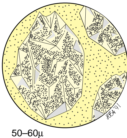
Figure 7-8. Schematic representation of the relation between filler particles and resin in conventional microfilled composites (eg, Isopast, Heliolit, Silar, Durafill, Silux, Silux Plus Filtek™ A110, and Renamel).
