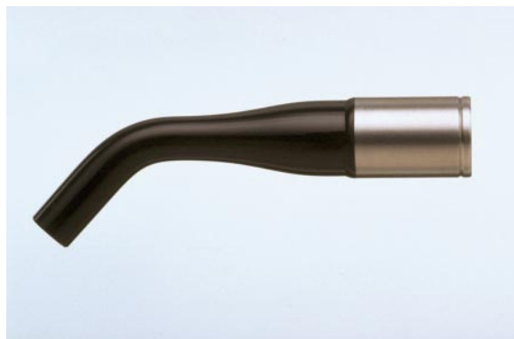
Figure 6–22. A Turbo light guide from Demetron. This unit reduces the diameter of cure but increases light intensity (by 34% on the Optilux 150 and by 50% on the Optilux 400 series curing lights). This increased intensity better activates the light portion of dual-cured resin cement.
