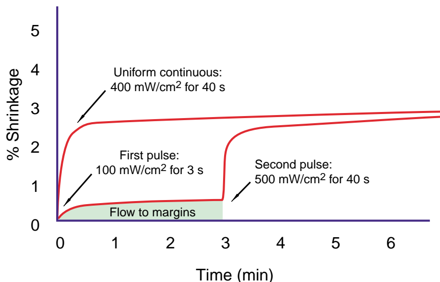
Figure 6–12. Plot of the typical reduction in strain from curing in two separate pulses over a 3-minute period. The first pulse is low energy to allow the composite to better remain attached to the margins. The second, delayed, pulse is high energy to complete the conversion of the composite. (Modified from information provided by Bisco, Schaumburg, Illinois.)
