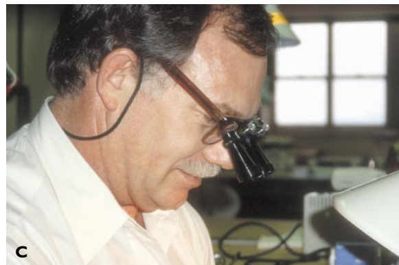
Figure C-5. A , Schematic of Greenough optics. B , Glasses-mounted Greenough lenses with adjustable magnification. C , Glasses-mounted Greenough lenses with fixed working distance and fixed magnification.
