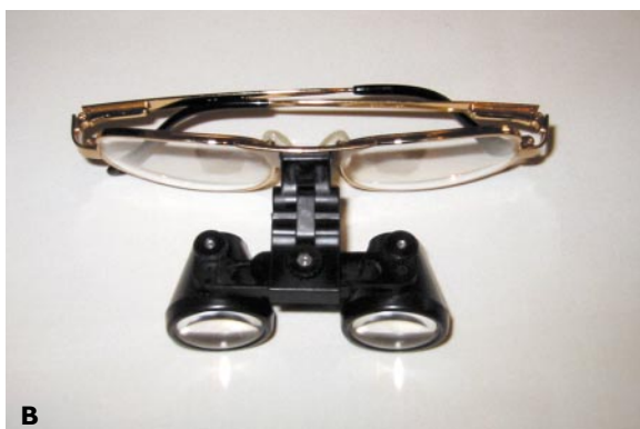
Figure C-4. A , Schematic of Keplerian optics compared to double-lens optics. Note that Keplerian optics result in transmission to the eye of an upright object; the object in two-lens optics is upside-down. B , Flip-up version of Keplerian-lens loupes. C , Keplerian lens mounted on glasses.
