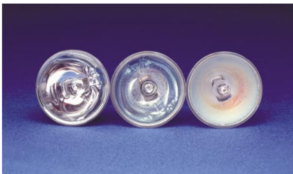
Figure 6–23. The bulb on the left is new and reads over 500 mW/cm 2 . The bulb in the middle is 3 months old and reads 240 mW/cm 2 . The bulb on the right is 9 months old and reads under 50 mW/cm 2 . All three lamps were used in the same curing unit 5 days a week. The bulb that reads 240 mW/cm 2 ( middle ) was used approximately 30 to 120 minutes per day for about 3 months. The bulb that reads under 50 mW/cm 2 ( right ) was used approximately 30 to 120 minutes per day over 1 year. Note that the bulb on the right shows most of the features associated with bulb degeneration.
