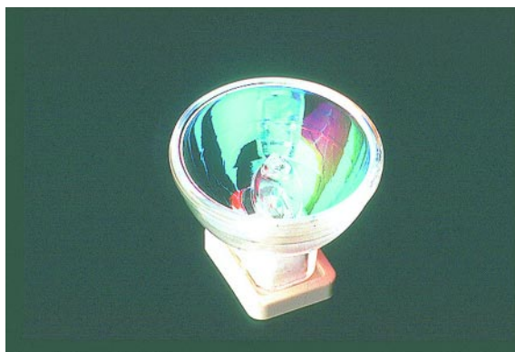
Figure 6–24. One of the newer curing bulbs that produce more 468-nm light. This bulb, from Demetron, also provides improved focus, better uniformity of light output, less energy consumption, and less heat production.
