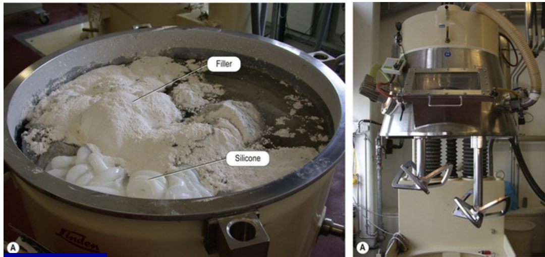
Fig. 15.24 (A) Vat of the contents of an addition silicone impression material prior to mixing. (B) The machine used to mix the material.
