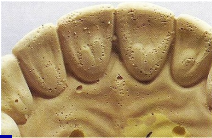
Fig. 15.25 Hydrogen gas released from an addition silicone impression material has caused porosity on the model surface as it has been poured too quickly.
