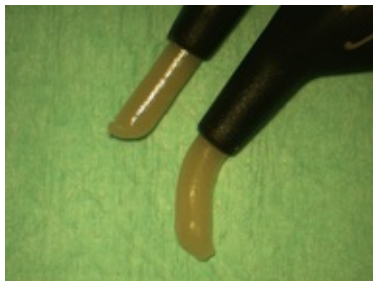
Fig. 5.5 Comparison between a resin composite stored in too cold a condition (upper compule) and another which is too warm. Note their different viscosities: the colder material is more rigid and the warmer one is more fluid.
