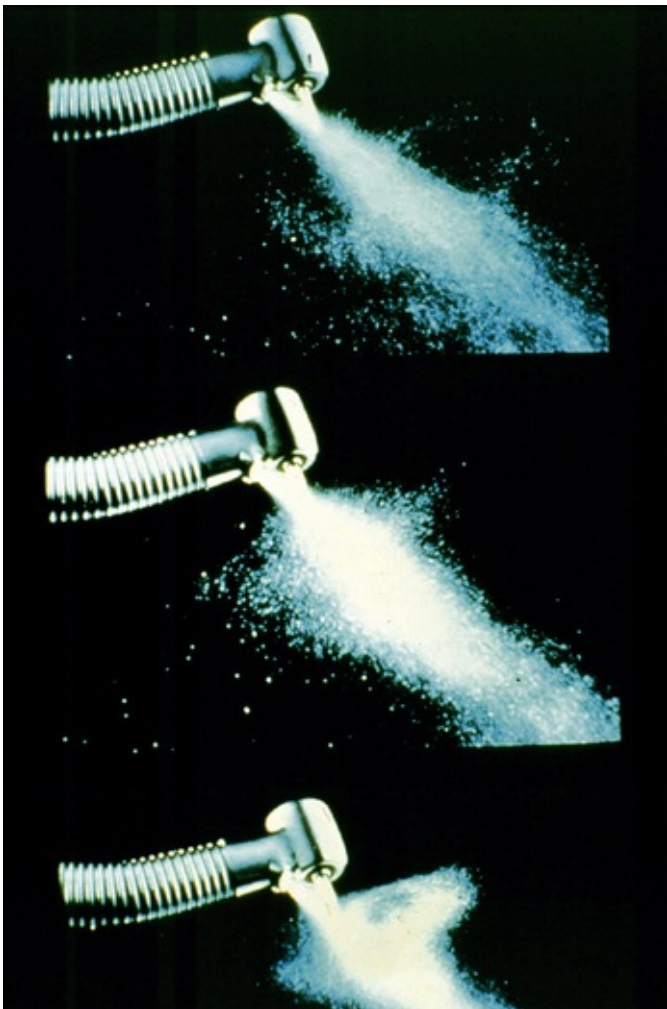
Fig. 19.7 The effect of water and air spray directed from the two apertures on the handpiece head simultaneously. Once air is incorporated, the water does not touch the bur at all. The water flow is disturbed and the air becomes the coolant, but this is ineffective in dissipating the heat.
