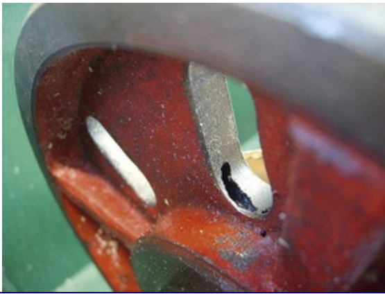
Fig. 21.23 An example of a blow hole defect in cast iron. This defect could have resulted in catastrophic failure with the fly wheel fracturing in service if it had not been detected.
