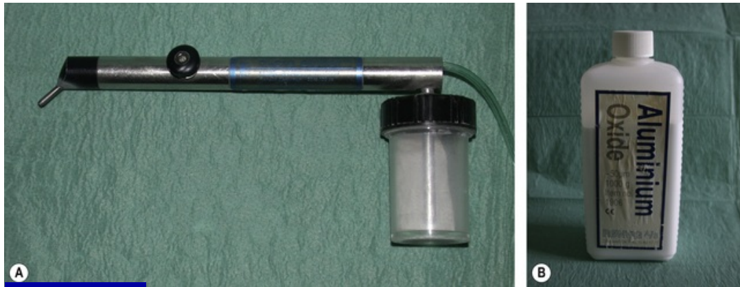
Fig. 19.36 (A) A sandblasting machine (Danville Engineering) which can be used extra- or intraorally. (B) It uses 50 \mu\text{m} alumina, which can be purchased separately.
