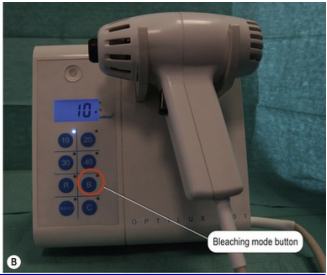
Fig. 18.11 Two lights which can be used in conjunction with a bleaching solution: (A) Zoom! Advanced Power (Discus Dental) and (B) Optilux 501 (Kerr), a high speed halogen curing lamp with a bleach mode.
