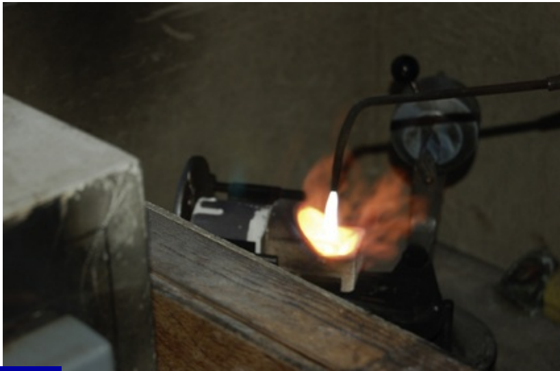
Fig. 21.18 Ingots of alloys being melted in the casting crucible by the application of heat from an oxyacetylene torch.
