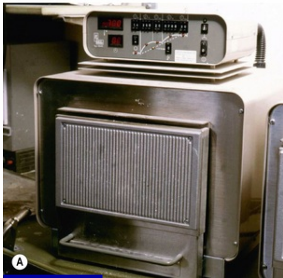
Fig. 21.17 (A) An oven used to burnout the wax pattern. (B) The oven door has been opened to show the casting ring inside.
