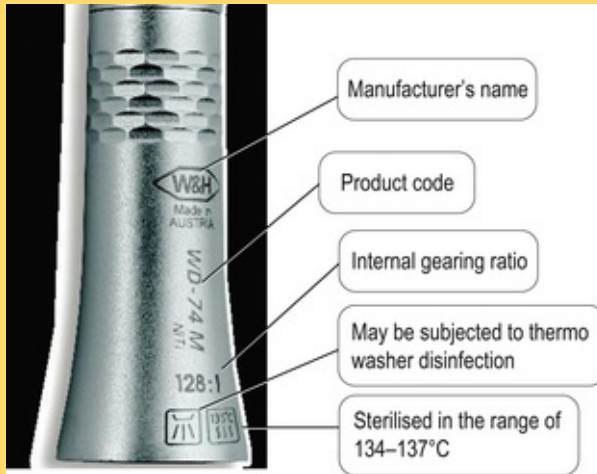
Fig. 19.20 External handpiece markings labelled with explanation of the codes.
