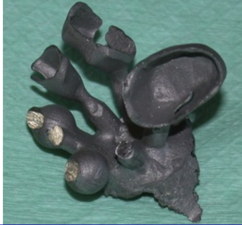
Fig. 21.24 A casting in which three of the seven patterns have not cast perfectly. Note the porosity and insufficient metal in these three remaining copings. (The other four copings have been removed from the button.)
