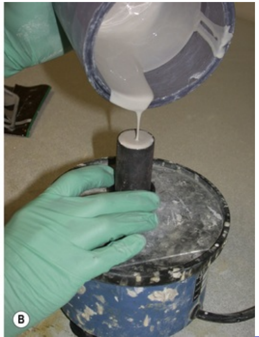
Fig. 21.16A,B The investment material is carefully poured into the casting ring on a vibrating base to ensure that no air is entrapped in the investment material or adjacent to the wax pattern.
