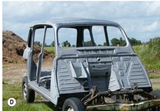
Fig. 19.32A–D (A) compressed air delivery system. (B) Abrasive (C) Nozzles for abrasive delivery (D) Finished surface after abrasion. The components and the technique for sandblasting metal work in industry. Note the protective equipment worn by the operator.
