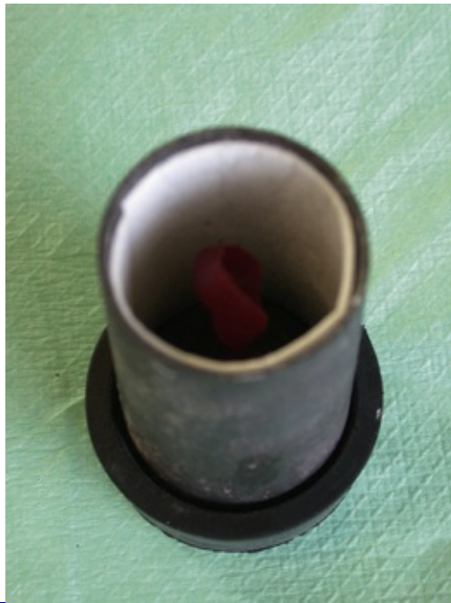
Fig. 21.15 The casting ring slid over the rubber base with the sprue and wax pattern placed in the centre of the ring to assemble the casting ring assembly.
