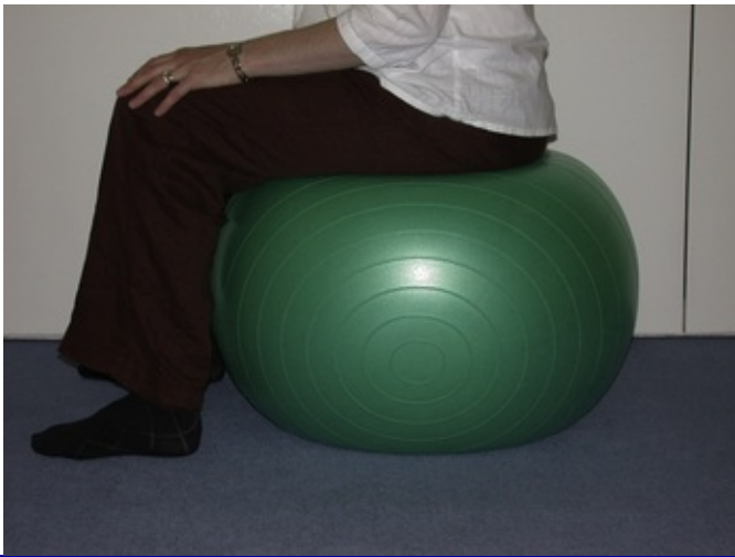
Fig. 4.6 An exercise ball under compression. Note distortion rather than fracture. Diametral tensile testing is unsuitable for materials of this type.
