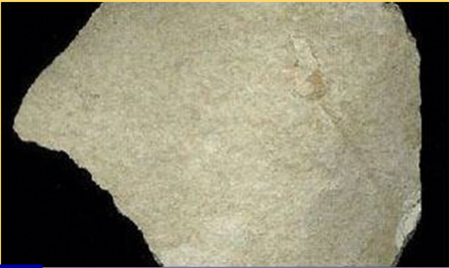
Fig. 15.15 Diatomaceous earth in its original form of soft siliceous sedimentary rock before being ground. (Photo courtesy of Minerály a horniny Slovenska) http://www.minerally.sk/
