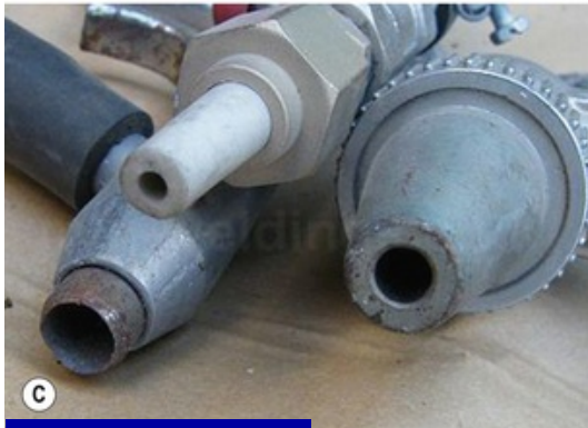
Fig. 19.32A–D (A) compressed air delivery system. (B) Abrasive (C) Nozzles for abrasive delivery (D) Finished surface after abrasion. The components and the technique for sandblasting metal work in industry. Note the protective equipment worn by the operator.
