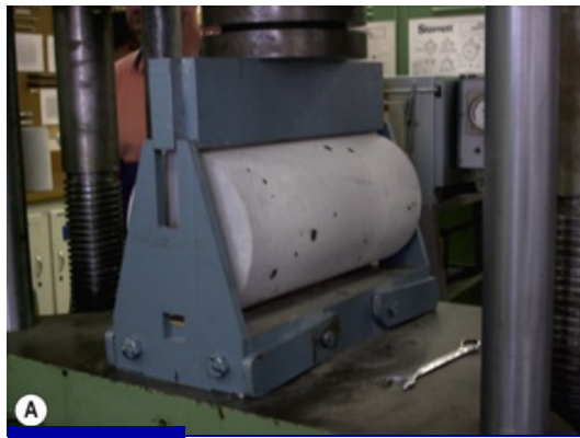
Fig. 4.5 A sample of Portland cement undergoing a diametral tensile strength test: (A) prior to loading and (B) after fracture.
