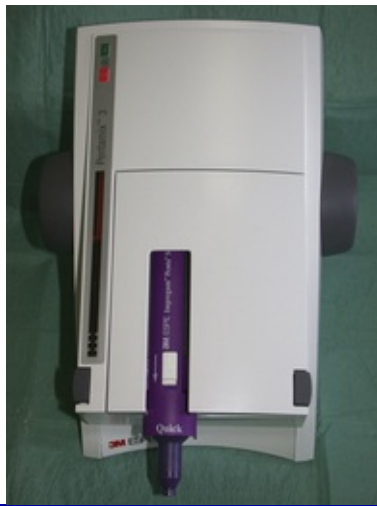
Fig. 15.35 Example of a mechanical mixing machine used to mix impression materials (Pentamix 3, 3M ESPE)
