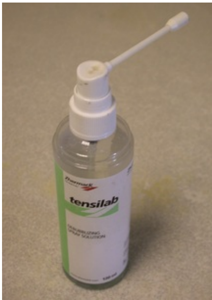
Fig. 20.21 A surfactant spray used to reduce the surface tension on a wax pattern prior to investing (Tensilab, Zhermack).
