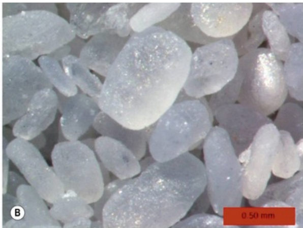
Fig. 20.1 (A) Gypsum stone as it occurs naturally. (B) A micrograph of the microscopic structure of the stone.
