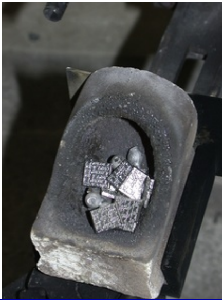
Fig. 21.22 The buttons from previous castings are being reused for a subsequent casting along with new ingots of metal.
