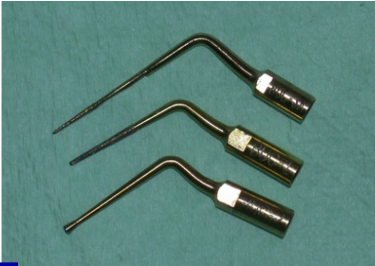
Fig. 13.42 A selection of zirconium nitride coated endodontic cutting tips used in an ultrasonic handpiece.
