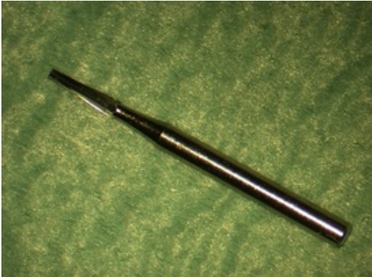
Fig. 19.3 A friction grip bur used with both high-speed and speed-increasing handpieces. Note the long smooth cylindrical portion of the bur, which is held in the jaws of the chuck by friction.
