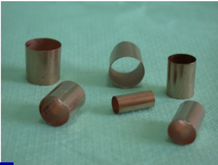
Fig. 21.26 A selection of copper bands which are supplied either hard (unannealed) or soft (annealed). The hard variety must be heated until cherry red before quenching in cold water. This will anneal them so rendering them malleable prior to use.
