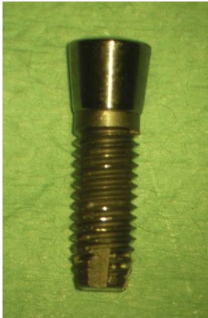
Fig. 17.38 A dental implant made from titanium alloy.
