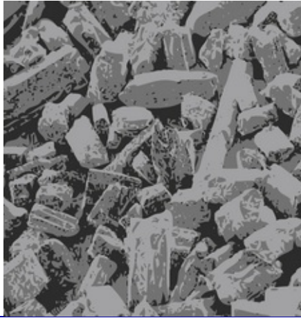
Fig. 20.6 Illustration of the crystal structure of die stone. Note the particles are much more uniformly shaped, smaller and denser than dental stone or plaster of Paris.
