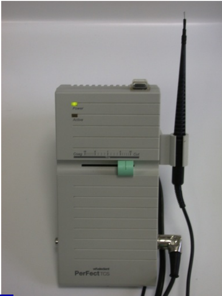
Fig. 15.49 Example of a dental electro-surgical unit that may be used to expose the margins of a preparation by removing the overlying gingival tissue (PerFect TCS, Whaledent).
