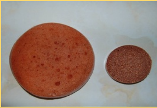
Fig. 4.14 Polymer disc before and after immersion in water for 6 hours, showing hygroscopic expansion due to water uptake and sorption.
