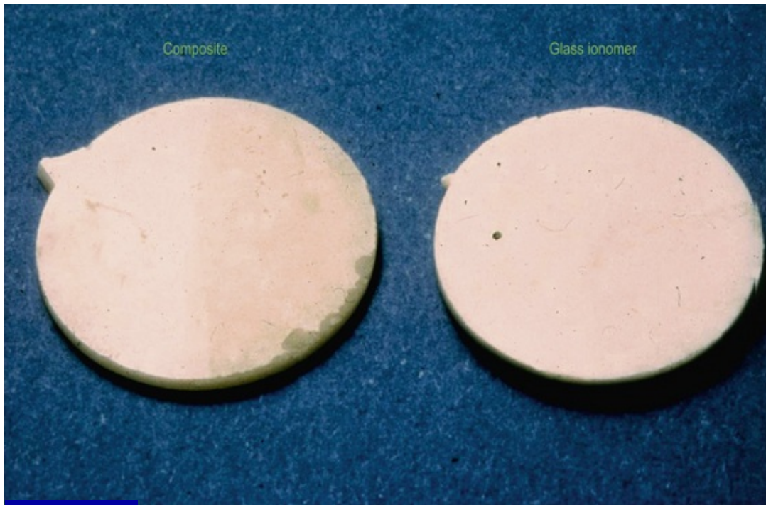
Fig. 9.16 Two discs of material: resin-based composite on the left and glass ionomer cement on the right. Half of each disc was protected by foil and the other half exposed to sunlight for 3 months. Note the marked change in colour on the composite disc, not observed with the glass ionomer sample.
