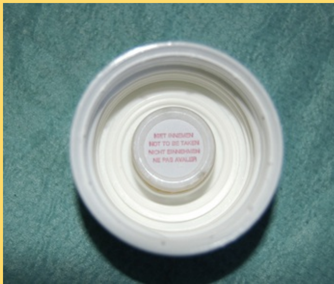
Fig. 9.19 The desiccant container in the lid of a bottle of glass ionomer powder.
