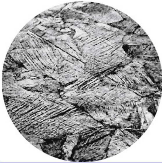
Fig. 21.25 Photomicrograph of a wrought alloy. Note its fibrous grain structure.
