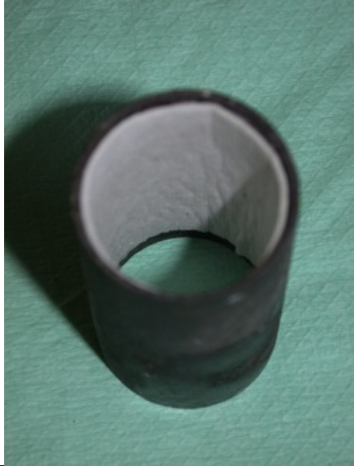
Fig. 21.14 The casting ring lined with a sheet of lining material to counteract the effects of expansion of the investment during the heating and cooling phases.
