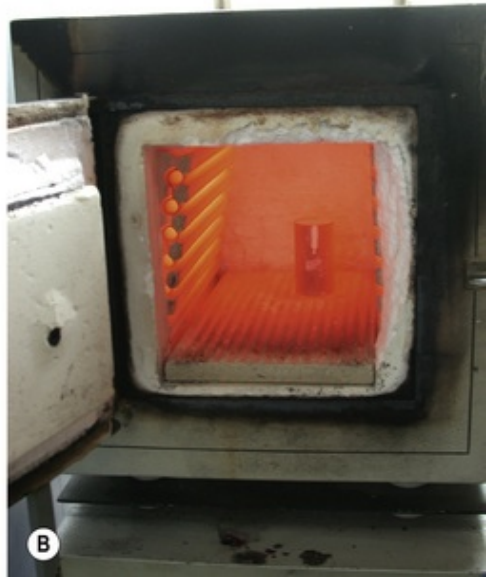
Fig. 21.17 (A) An oven used to burnout the wax pattern. (B) The oven door has been opened to show the casting ring inside.
