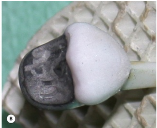
Fig. 21.8 (A) A metal coping forming the substructure for a metal ceramic crown just prior to the placement of the ceramic on the buccal surface. The design of the coping allows the ceramic to shrink fit onto it. Note also the grey matt surface (caused by sandblasting) to afford some micromechanical retention for the ceramic to bond to the metal. (B) The same coping with the ceramic fired on to it.
