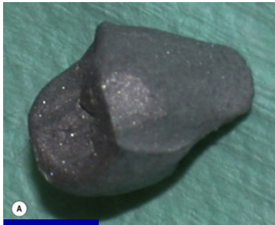
Fig. 21.8 (A) A metal coping forming the substructure for a metal ceramic crown just prior to the placement of the ceramic on the buccal surface. The design of the coping allows the ceramic to shrink fit onto it. Note also the grey matt surface (caused by sandblasting) to afford some micromechanical retention for the ceramic to bond to the metal. (B) The same coping with the ceramic fired on to it.
