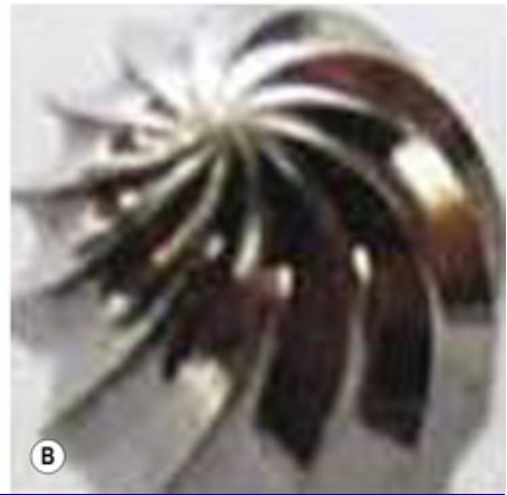
Fig. 19.26 Magnified images of two tungsten carbide burs. (A) A friction grip bur for use with a high-speed handpiece and (B) a bur used in a straight handpiece for trimming acrylic.
