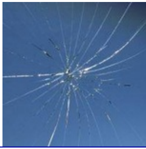
Fig. 4.12 A sheet of glass that has been subjected to a load, causing it to fracture. The force applied therefore rises quickly to a point where the glass breaks. This is explained in Figure 4.11 .
