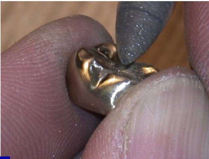
Fig. 21.21 The casting with the sprue removed being ground and polished to a high lustre.
