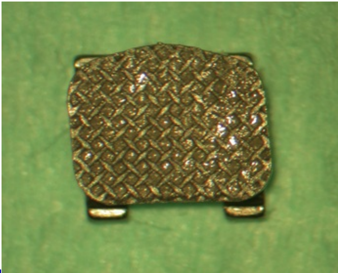
Fig. 11.28 Stainless steel orthodontic bracket that will be bonded onto the tooth surface using resin composite. Note the mesh, which will aid the micromechanical retention with the resin composite.
