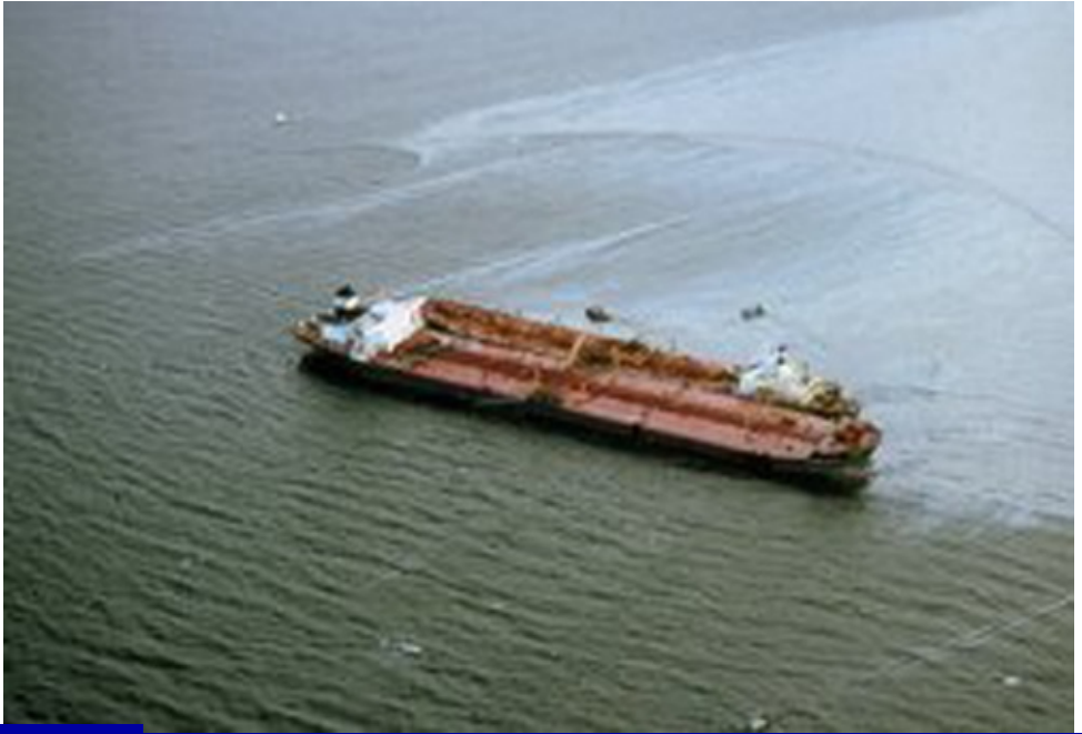
Fig. 11.4 Oil spill from the Exxon Valdez showing the effect of surface tension with the oil on top of the water.
