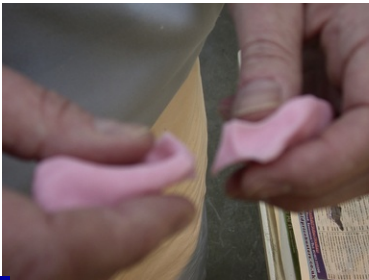
Fig. 23.8 Acrylic dough at the snap stage. Note the clean separation of the material when pulled apart.
