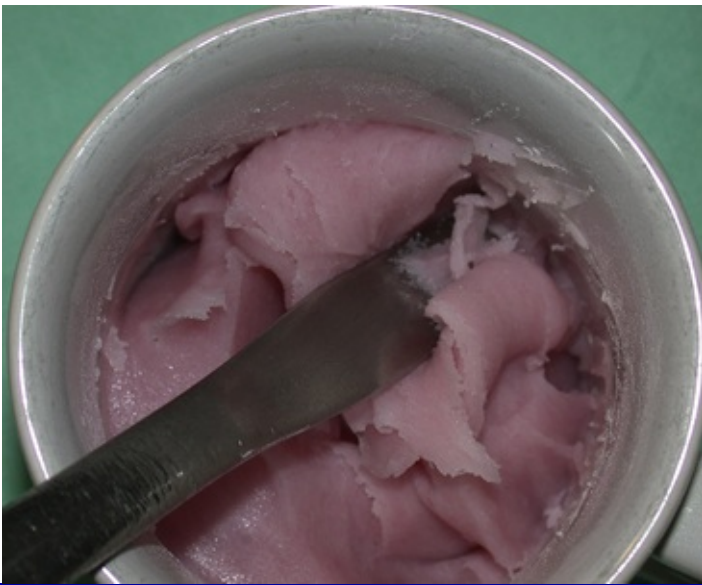
Fig. 23.7 Acrylic left undisturbed after mixing.
