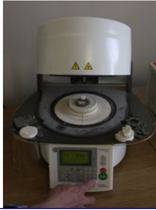
Fig. 22.6 A furnace used to bake dental ceramic. Note that the ceramic mass in the green state is sitting a short distance to the furnace entrance to allow water to be slowly driven off before it turns into steam. If steam was allowed to form, the powder core would break.
