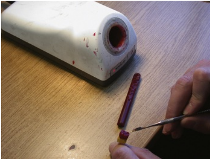
Fig. 16.7 The dental technician using an induction coil to maintain the correct temperature of the wax when a wax pattern is being made so that it can be manipulated effectively.
