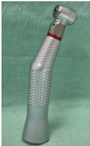
Fig. 19.2 A speed-increasing handpiece (Bien Air). Note the red ring on the proximal end of the instrument. This denotes that the internal gears increase the speed of the instrument.
