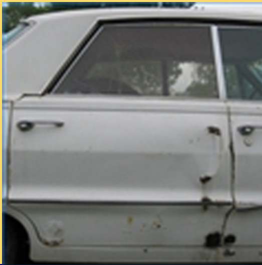
Fig. 4.16 Corrosion to the lower doorsill of a car as a result of water becoming trapped within the door frame and in the presence of oxygen starting a corrosion cell.
