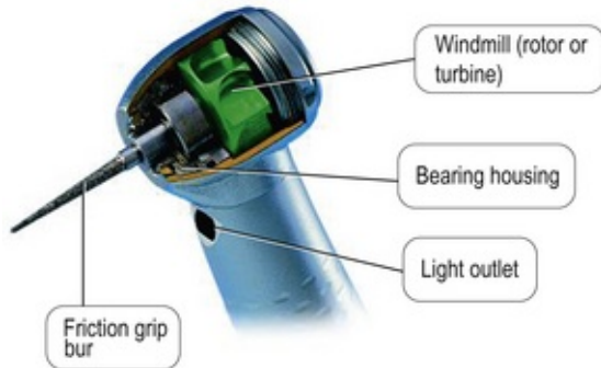
Fig. 19.5 The head of a high-speed handpiece with its components labelled. The blades of the windmill are driven by the compressed air.
