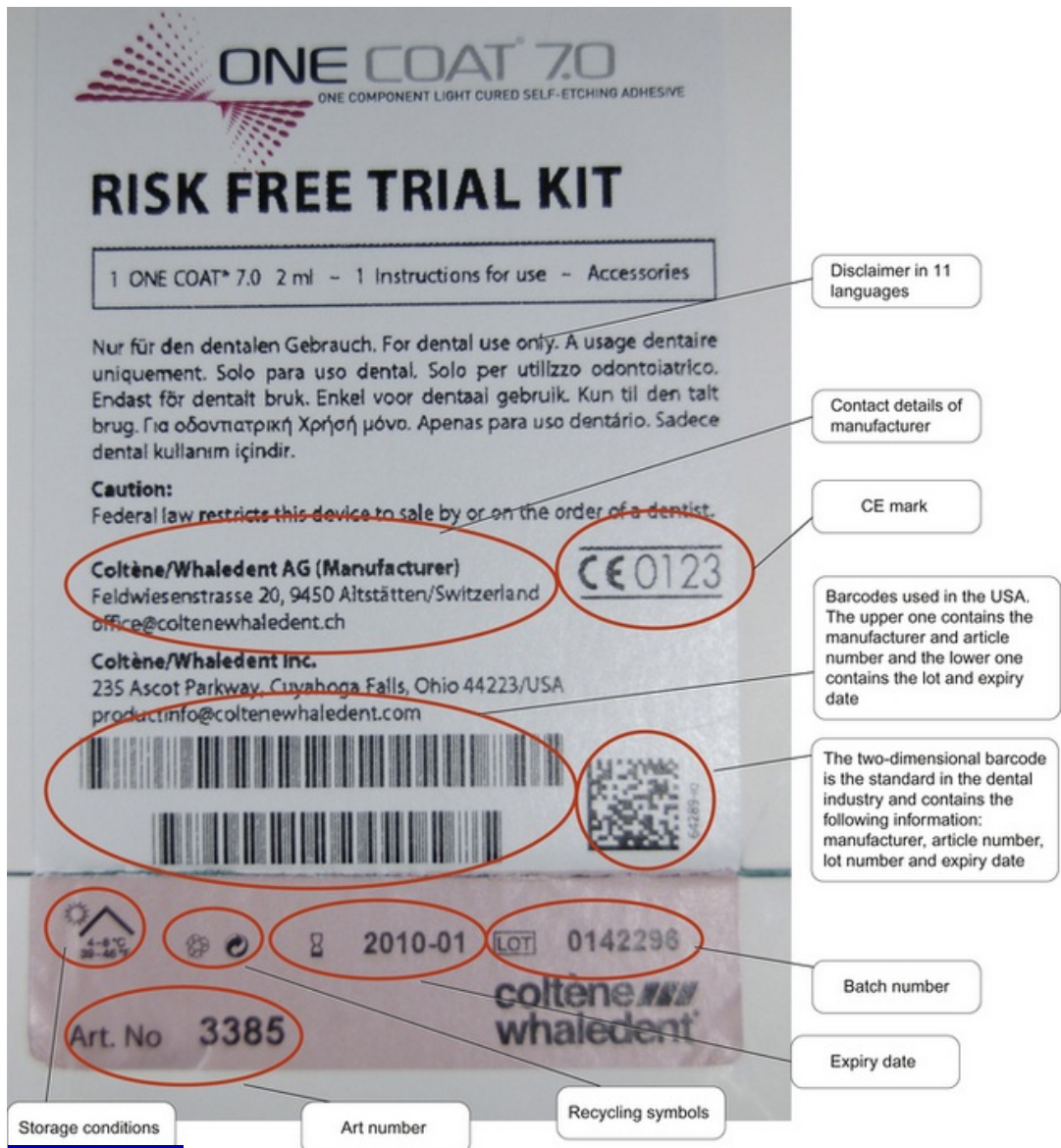
Fig. 4.24 The various warning labels found on dental materials and equipment.
