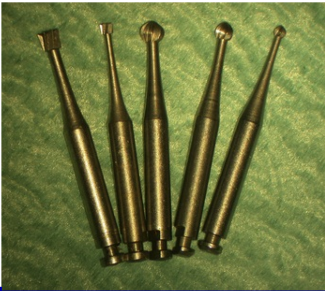
Fig. 19.30 A selection of stainless steel burs. The two burs on the left are two sizes of inverted cone burs while the others are round burs, again three sizes are shown.
