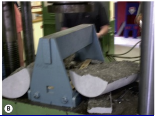
Fig. 4.5 A sample of Portland cement undergoing a diametral tensile strength test: (A) prior to loading and (B) after fracture.
