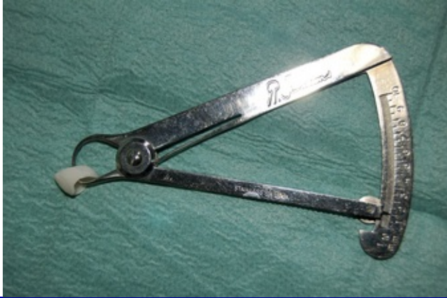
Fig. 14.1 An Iwansson gauge being used to measure the thickness of the occlusal surface of a indirect restoration, in this case a temporary crown.
