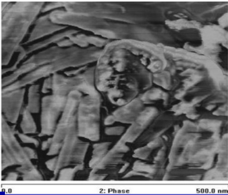
Fig. 13.3 Photomicrograph from atomic force microscopy showing the platelet-type layered structure of hectorite.
