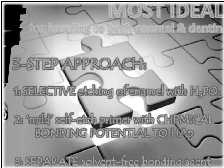
Figure 1.35 The most ideal adhesive approach today to durably bond to enamel and dentin according to KU Leuven BIOMAT.
