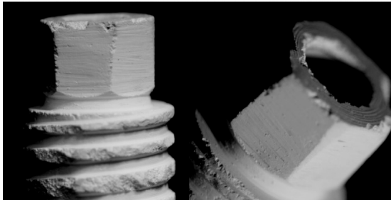
Figure 14.2 Direct milling and shaping of fine implant threads does not produce expected accuracy compared to machined titanium.
