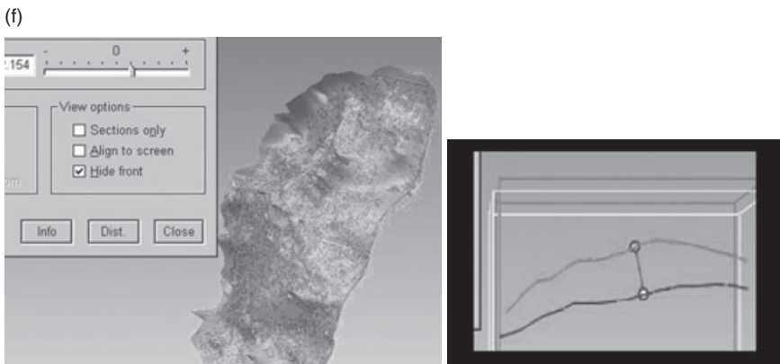
6.6 (d) Contour map. (e) Left-shell modeled surface for image in (a), while the right shell represents the image in (c); arrows in both images show the worn areas after 24 months. (f1) Cross-section of superimposed shells; distance between the two lines (f2) represents the depth of wear in the measured area.
