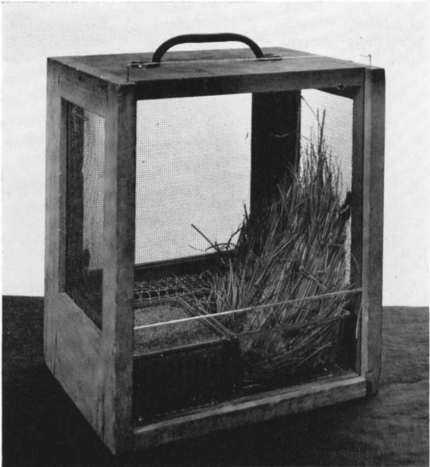
FIG. 2. Grasshopper cage. Shown are raised hardware cloth platform and dishes containing wet sand for egg-laying and water to keep leaves fresh.
