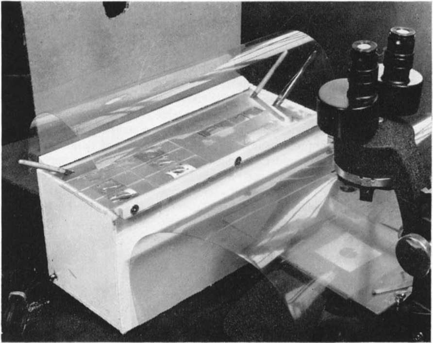
FIG. 5. Dissecting microscope equipped with rectangular glass plate to enlarge the stage, and plastic dust shield to decrease chance of contamination during manipulation of embryo in culture media. Aluminum cover of ultraviolet sterilization box shows openings for instruments, slides, and cover glasses. Cover with dust shield lifts off box (from Carlson et al. , 1947).
