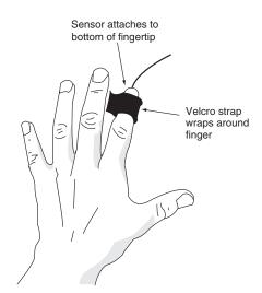
Figure 7.14 Pulse transducer for Biopac system.
