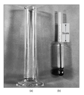
Figure 9.3 Instruments for determining the specific gravity of urine. (a) A glass cylinder and (b) a urinometer float.
