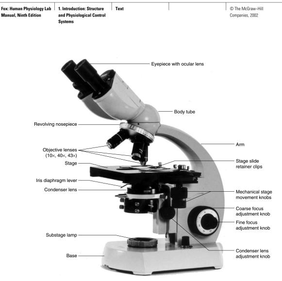
Figure 1.1 The parts of a compound microscope.
