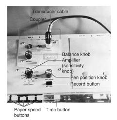
**Figure 5.3** The Narco Mark III Physiograph with an inserted transducer coupler. The transducer coupler is connected by means of a cable to a myograph transducer.
