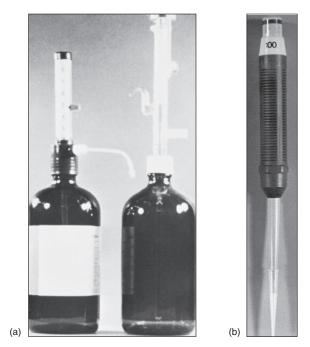
Figure 2.1 Automatic devices for dispensing fluids.
