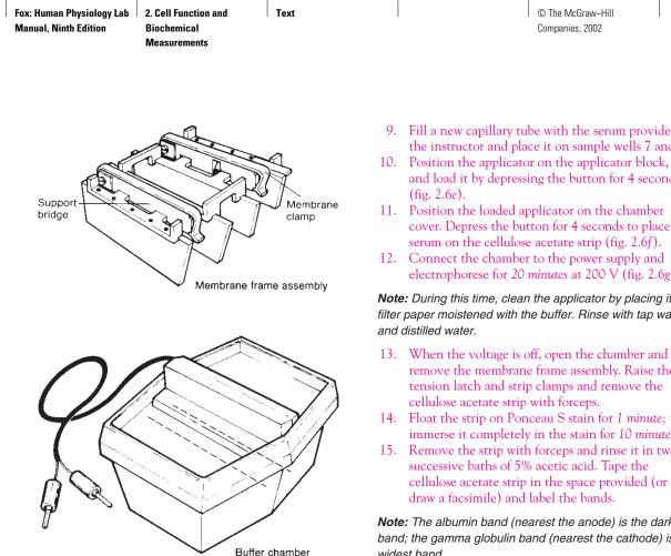
Figure 2.5 An electrophoresis system. A membrane frame assembly and buffer chamber for the Gelman Sepra Tek electrophoresis system.
