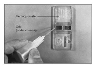
**Figure 6.4 Procedure for filling a hemocytometer.** A Unopette reservoir is used to fill the hemocytometer with diluted blood. The squeezing of the reservoir places a drop of diluted blood at the edge of the coverslip, whereupon the drop of blood moves under the hemocytometer grid by capillary action.
