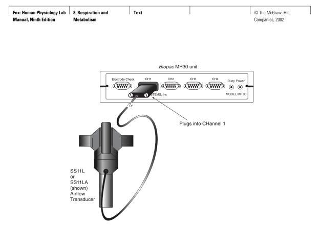
Figure 8.3 Biopac system equipment for spirometry.
