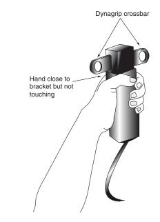
Figure 5.11 The Biopac hand dynamometer.
