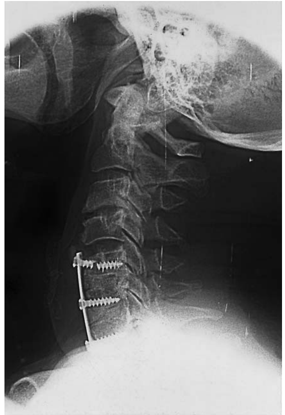
Fig. 4.49 - Fracture of surgical spinal appliance. A lateral radiograph of the cervical spine shows a fracture of the upper vertebral body screw in a patient with cervical myelopathy operated on for spinal cord decompression and anterior fusion.
