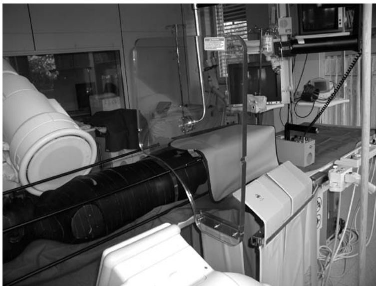
Figure 4b.8 Optimized table-attached radiation protection with closure of radiation leakage between overcouch and undercouch lead protection devices and a lead cover around the patient's thighs.
