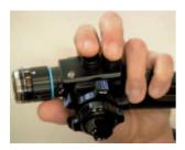
**Fig. 5.2** Approach to the air/water and suction buttons. The index and the ring fingers are free to work with the air/water and suction buttons.
