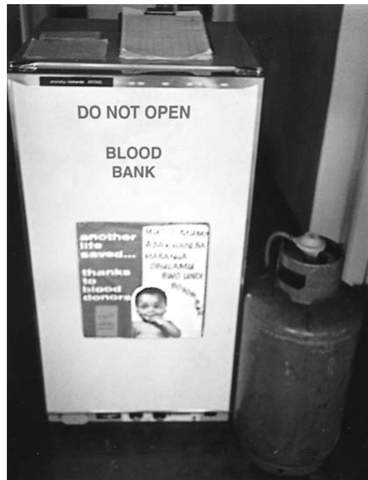
Plate 9.3 Thermostatically controlled gas operated refrigerator for storing blood in a district hospital.
