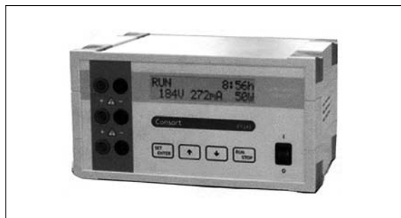
Plate 8.9 EV 243 Power Supply suitable for cellulose acetate haemoglobin electrophoresis with integral digital timer.
