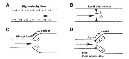
Causes of turbulence. In **A**, turbulence occurs in fluids flowing at high velocity through tubes of uniform caliber, according to the formula for Reynolds numbers. In **B** and **C**, either a local obstruction or fluid flowing into a channel of larger diameter can produce turbulence at much less flow velocity. In **D**, a combined effect of obstruction and abrupt increase in caliber, as in poststenotic dilatation, produces turbulence at relatively low flow velocity.
