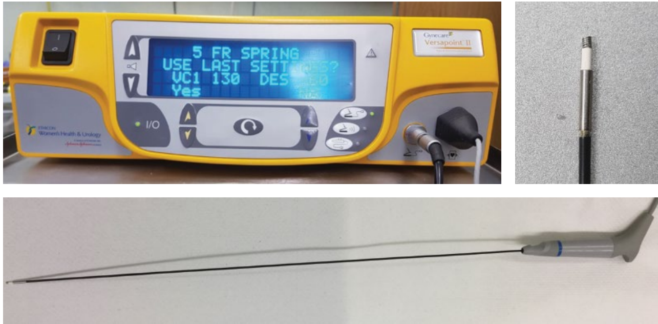
Fig. 37.3 Versapoint Bipolar Electrosurgery System™ (Ethicon, USA). Spring-tip electrode suitable for removing polyps, and grade 0 fibroids) is shown with the electrosurgical generator. A needle-like twizzle-tip electrode is also available (not shown) for removing polyps, septa, and adhesions. Source: photos by T. Justin Clark.
