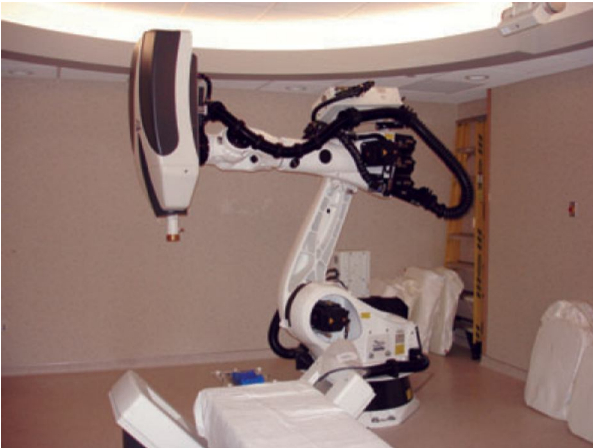
Figure 121-17 CyberKnife Robotic Radiosurgery system manufactured by Accuray, Sunnyvale, CA.
