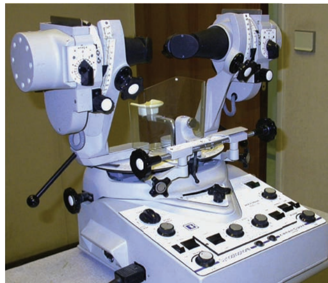
FIGURE 26.5 Synoptophore: Binocular viewing device that can be used to determine fusion ability of individuals with diplopia who have had long-standing severe monocular visual loss in which the vision has been restored (e.g. correction of aphakia). (From Oystreck DT, Lyons CJ. Saudi Journal of Ophthalmology 2012;26(3):265–270)
