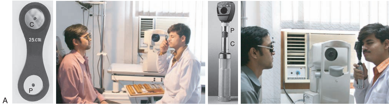
FIGURE 7.1 (A) Left: Mirror retinoscope: C, concave mirror; P, plane mirror. Retinoscopy being performed with a mirror retinoscope. Right: Streak retinoscope. Retinoscopy being performed at 1 m distance with a self-illuminating streak retinoscope which functions similar to a concave mirror with the lens adjustment sleeve in position C and plane mirror in position P.
