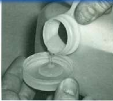
Fig. 9-64. Tinfoil substitute is poured in small container for immediate use. Any tinfoil substitute remaining after using should be discarded and not returned to storage container.
