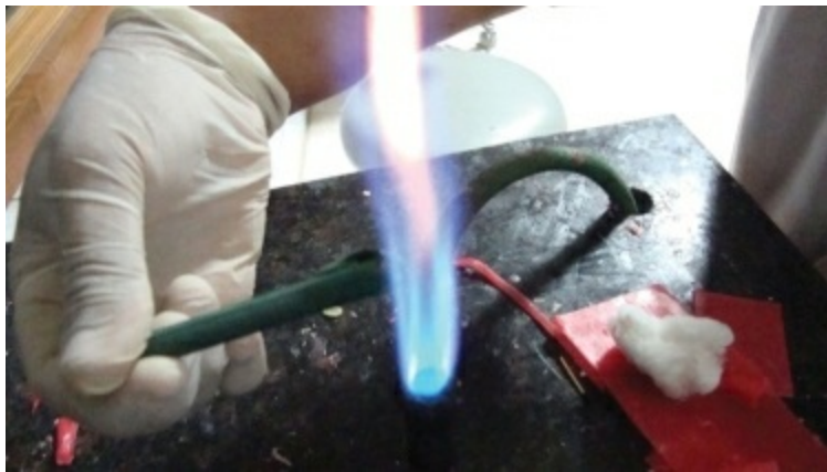
FIG 1.1.12.10 Tracing compound softened over a flame.
