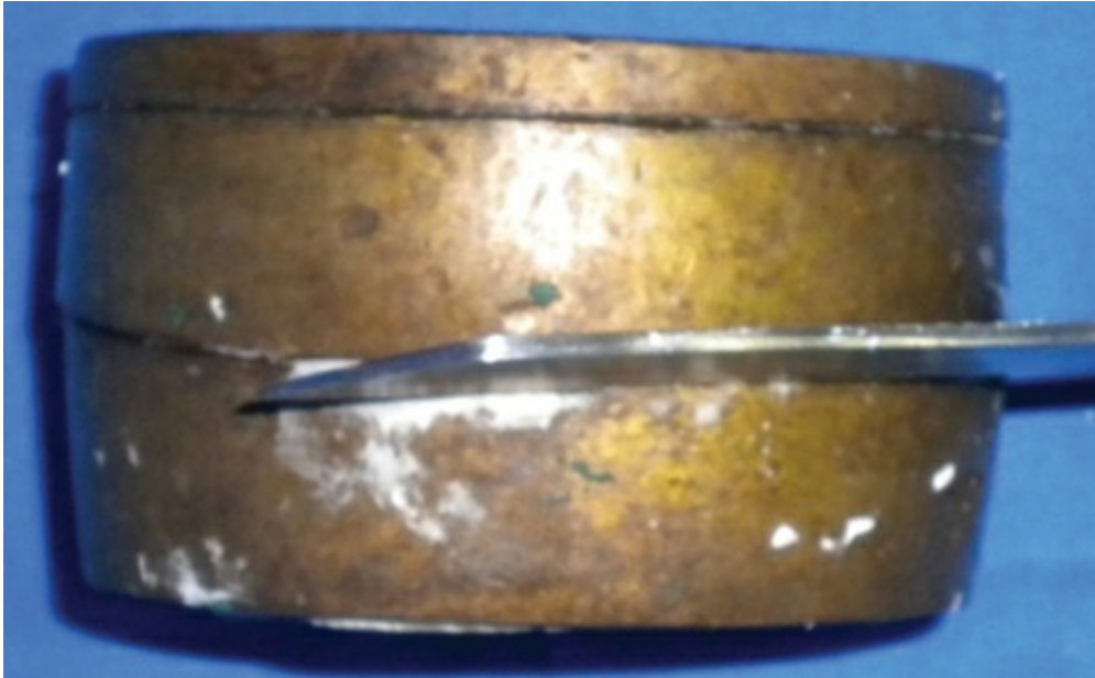
FIG 3.1.8.3 Separation of the upper and lower halves of the flask.
