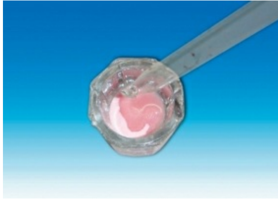
FIG 3.2.15 Manipulation of repair resin.
