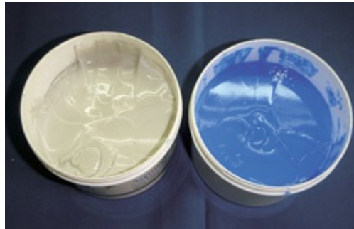
FIG 2.2.11 Addition silicone – putty consistency.
