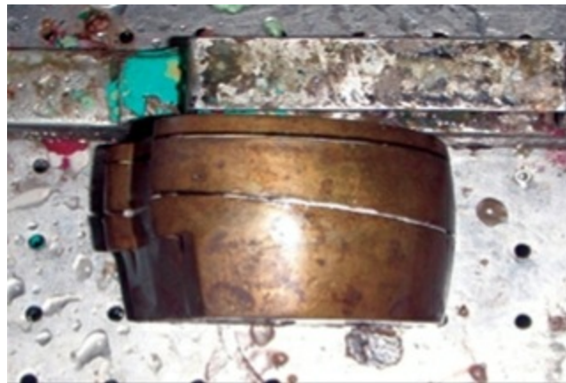
FIG 3.1.7.28 Upper flask placed in the dewaxing tray.
