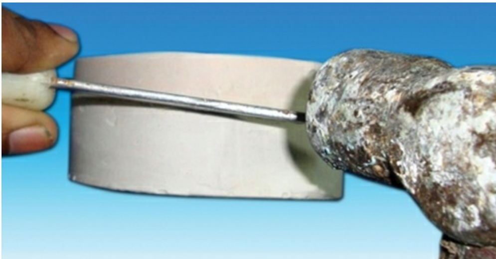
FIG 3.1.8.4 Removal of stone.
