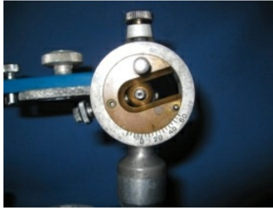
FIG 1.1.8.4 Condylar sphere in the upper member and condylar track in the lower member.
