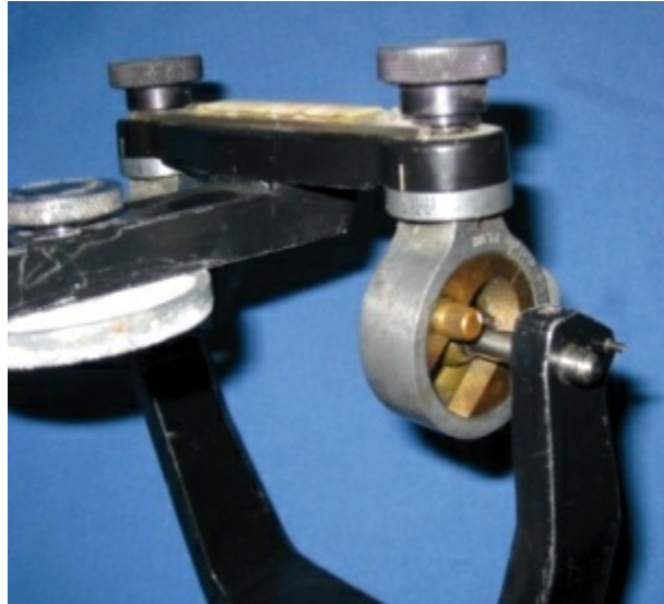
FIG 1.1.8.2 Condylar guidance in the upper member and condylar spheres in the lower member.
