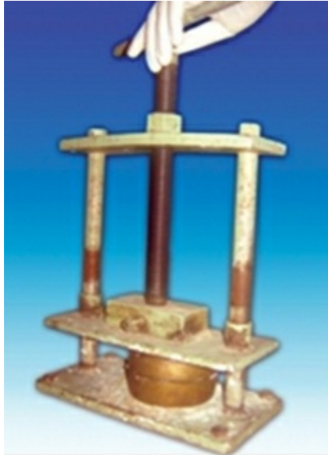
FIG 3.4.8.18 Final closure of the flask after packing.
